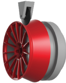
Roller presses onto blank and begins to mold wheel
